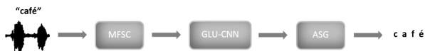
Figure 1: Architecture of the end-to-end ASR system based on Wav2Letter system. Adapted from [17].
