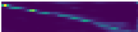
Figure 2: Dot-product attention from LAS model. The x-axis represents input frames, and the y-axis corresponds to output labels (row i corresponds to the i -th label). Larger values appear yellow, and lower values appear purple.
