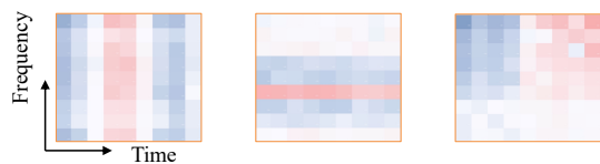
Figure 2: Examples of 9 \times 9 filters after cross entropy training in the first convolutional layer (best viewed in color). Red and blue represent positive and negative values, respectively.
