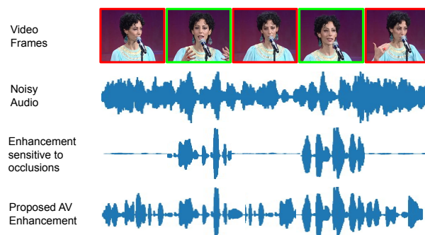
Figure 1: An audio-visual speech enhancement model may fail when the lip region is occluded by e.g. a microphone. In such cases the input audio is often entirely filtered out and the result is silent output over the occluded frames. The aim of our method is to be robust to this kind of occlusions.
