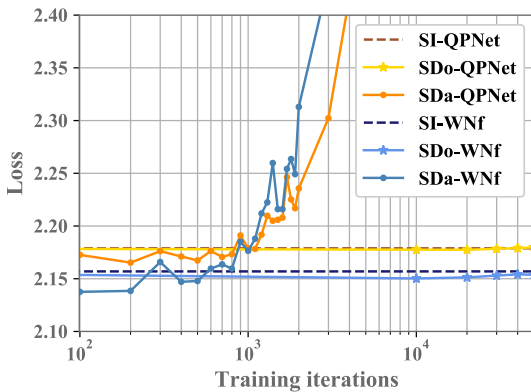
Figure 5: Validation losses of different vocoders (SI: speaker-independent; SD: speaker-dependent; o: only update output layers; a: update whole network)
