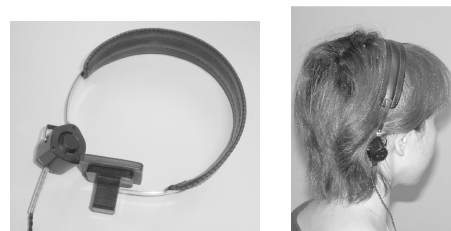
Figure 1: Ceramic vibrator of the BCUHA attached to the mastoid with a hair band-like device
