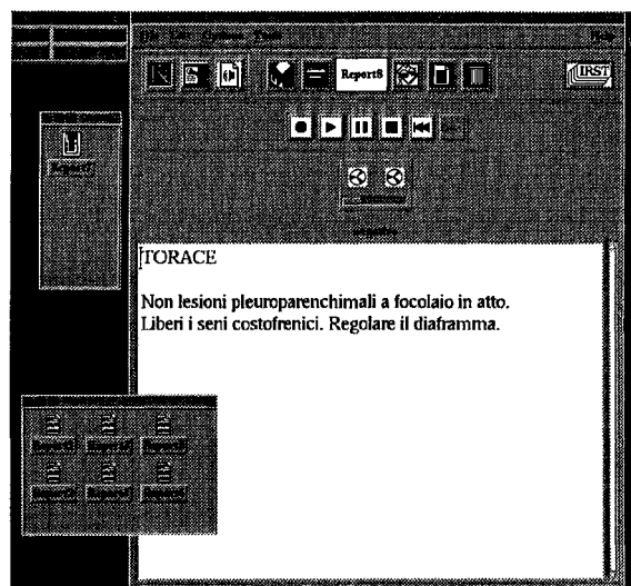
Figure 2: Graphical User Interface. It consists of three windows: the main window, with the digital voice recorder and the word processor, the window of the cassette queue (top left) and the window of completed reports (bottom left).
