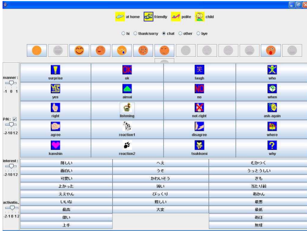
Figure 3: The Chakai Conversational Speech Synthesis interface. By clicking on a speech-act icon, a choice of emoticons is displayed in the upper section of the screen according to corpus availability, from which an utterance having the appropriate speech characteristics can be selected. Utterances are selected at random from among those in that same category within the corpus so that subsequent selection of the same combination will provide natural variety without unnecessary repetition.
