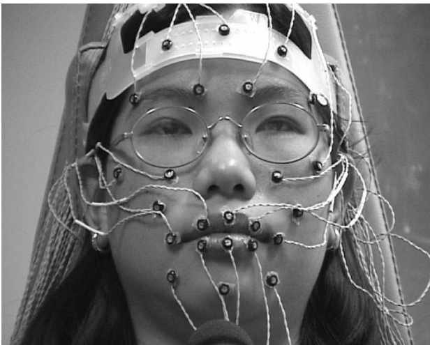
Figure 1: Positions of Optotrak markers in the speaker's face. The microphone was positioned under the chin. The head rig was used for capturing rigid head movements.
