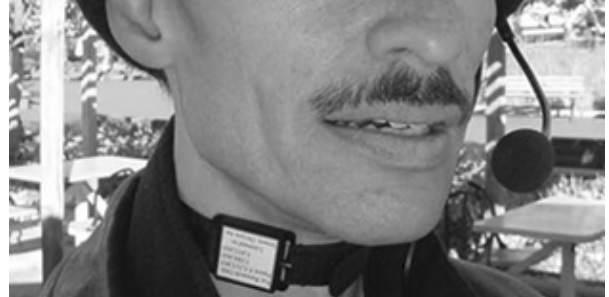
Figure 5. Speaker Set-up, A-MIC and P-MIC
