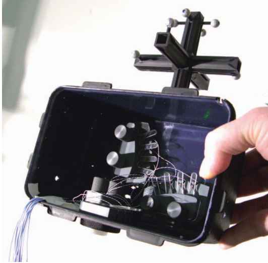
Figure 2: Inside of the custom-built container showing the three EMA calibration cartridges
