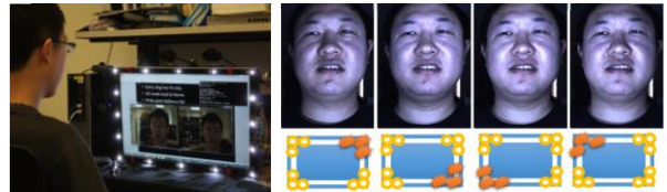
Fig. 2: Left is a recording scene. Right are four adjacent frames captured by one camera, with their corresponding LED lighting patterns at the bottom.
