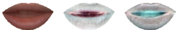
Figure 2: The mean and first three modes of variation of the appearance component of an AAM. The appearance images have been suitably scaled for visualisation.
