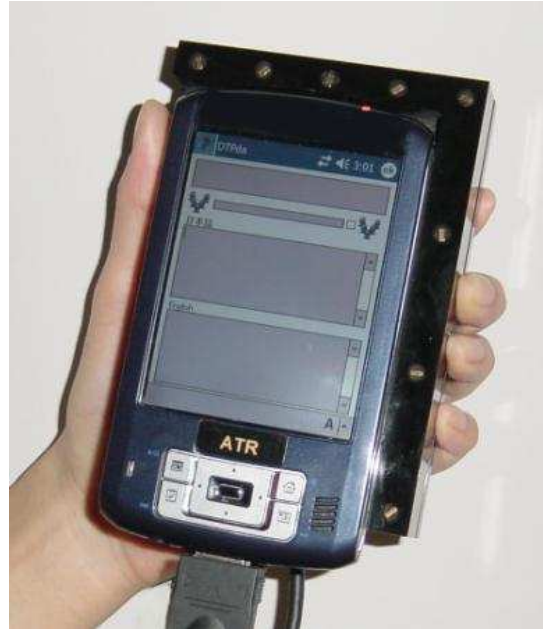
Figure 2. Mobile multi-channel speech input device with PDA terminal. Eight microphones are arranged as reverse L-shaped array.
