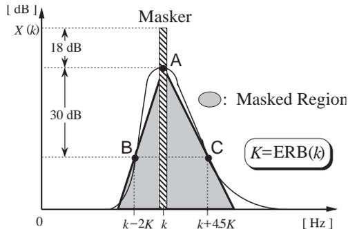
Figure 1: A masking pattern as an approximation of the masking pattern for narrow-band noises measured by Egan and Hake.
