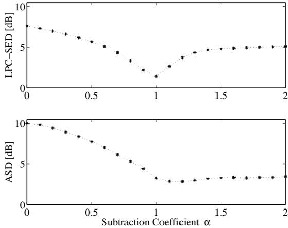
Figure 5: Distortions on the LPC-SED and the ASD of noise-reduced speech signals for each subtraction coefficient  $\alpha$ .
