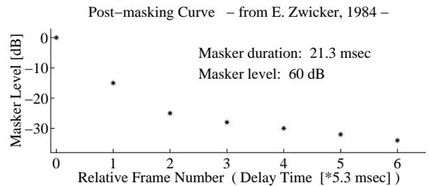
Figure 2: A post-masking curve measured by Zwicker.
