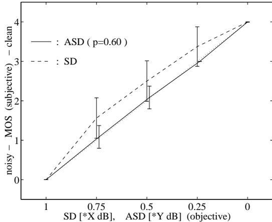
Figure 3: An interrelated curve between the ASD(a solid line) and the SD(a broken line), and the MOS.
