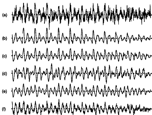
Figure 2: Reduced noise speech estimates, (a) noise corrupted vowel /r/, (b) clean speech, (c) time series A, (d) series B, (e) series C, (f) series D.
