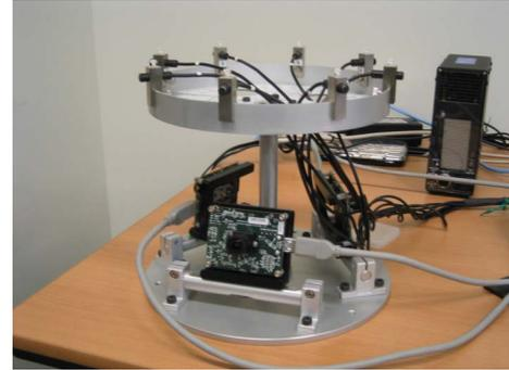
Figure 4.1 Microphone array and camera array used for the recording.
