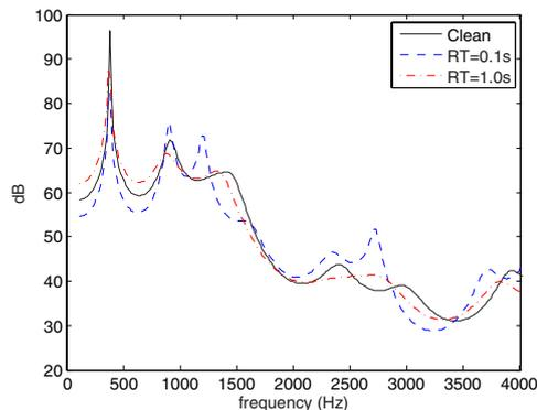
Figure 3: Comparison of 16<sup>th</sup> order LP spectral envelopes for clean (solid) and reverberant speech with  $RT = 0.1$ s (dashed,  $SD = 4.5$ dB) and  $RT = 1$ s (dot-dashed,  $SD = 2.5$ dB).
