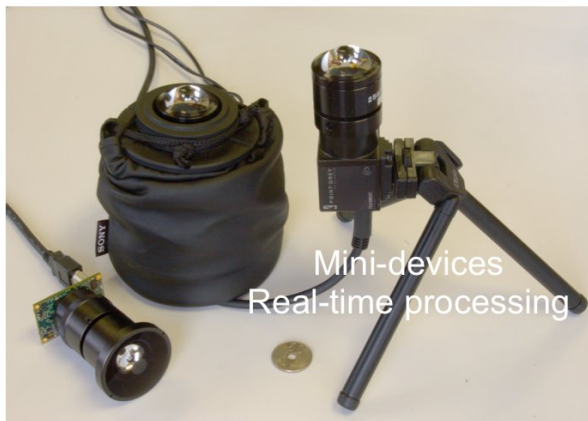
Figure 1: The 360-degree lens assembly taken from a SONY RPU-C251 device (left), and fitted to a PointGrey Flea2 industrial video camera (right) and a similar Palnon lens on a small firewire Firefly camera (bottom left).
