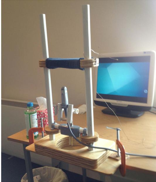
Figure 1: *The adjustable-height head-rest/probe-holder*
