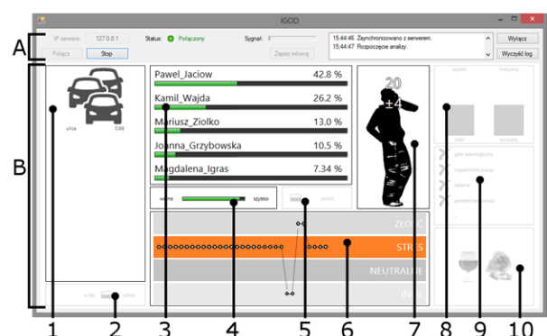
Figure 1: System GUI: A – communication panel, B – results panel (1 – acoustic background, 2 – language in the background, 3 – identity, 4 – speech rate, 5 – language, 6 – emotional state, 7 – gender and age, 8 – physical features, 9 – voice characteristics, 10 – degree of intoxication).
