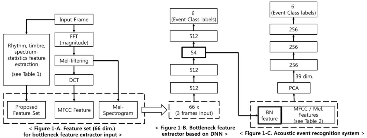
Figure 1: Proposed acoustic event recognition framework based on bottleneck features.
