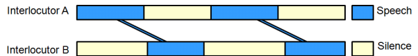
Figure 2: Illustration of setting up dialog turn pairs. Dyadic synchrony is computed for each pair of dialog turns.
