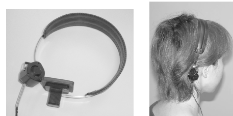
Figure 1: Ceramic vibrator of the BCUHA attached to the mastoid with a hair band-like device
