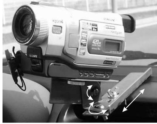
Figure 6: *Details of the directions of camera movements.*
