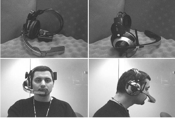
Figure 1: *First row: frontal and side view of the infrared headset; Second row: frontal and side view of a subject wearing the headset.*
