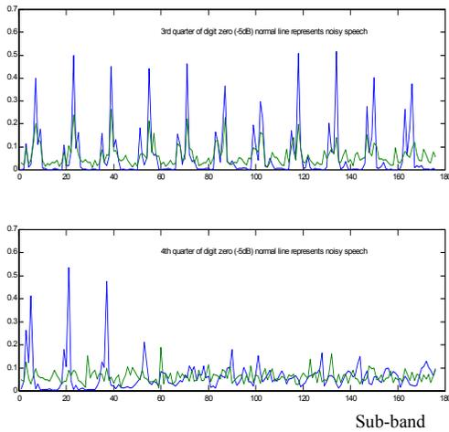
Figure 2. White noise effect in the power spectrum density normalization domain in a voiced segment (upper part) and in an unvoiced segment (last 2/3 of the lower part of the figure). Dashed line represents noisy speech features.
