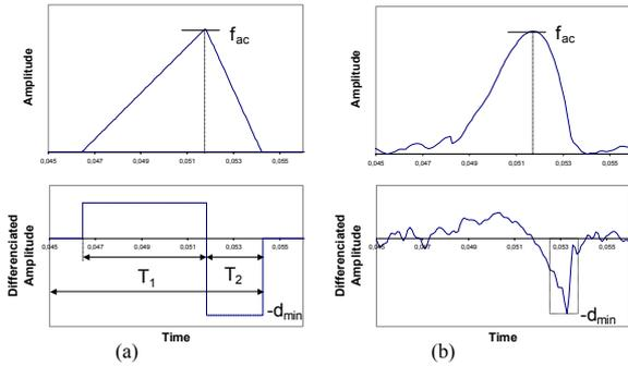
Fig.1. Definition of the NAQ. (a) Triangular-shaped glottal flow pulse. (b) Natural speech inverse filtered glottal source excitation
