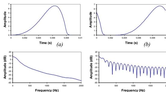
Fig. 5. (a) Glottal source FFT spectrum for a right period selection. (b) Glottal source FFT spectrum for a wrong period selection
