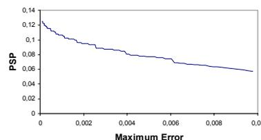
Fig. 6.a. Dependence of the PSP on the maximum error
