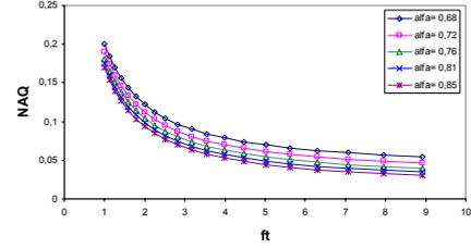
Fig 3.b. NAQ versus normalized cut-off frequency of the Spectral Tilt.  $O_q=0,2$
