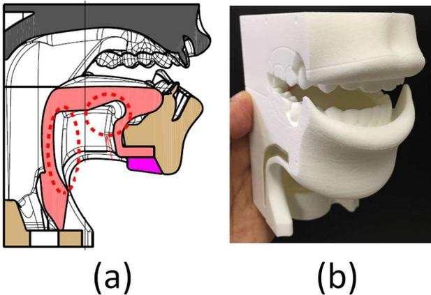
Figure 3: (a) Mid-sagittal cross-section of the proposed model. (b) Photograph of a prototype.
