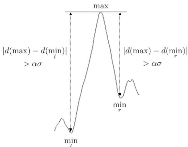
Figure 4: A significant max in the distance curve.
