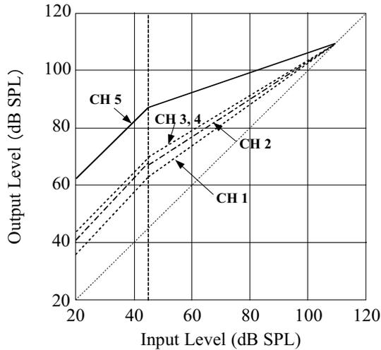
Figure 4: Input-Output level functions.
