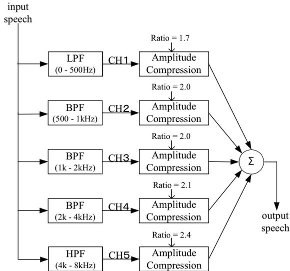
Figure 2: Block diagram of WDRC (multi-band amplitude compression). CH5 exists only in wide band condition.
