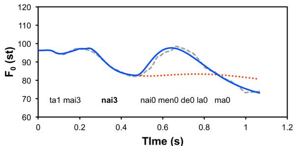
Figure 2: Examples of  $F_0$  contours synthesized with (solid blue) and without (dotted red) post-L bouncing simulation, together with the original  $F_0$  contour (dashed gray).
