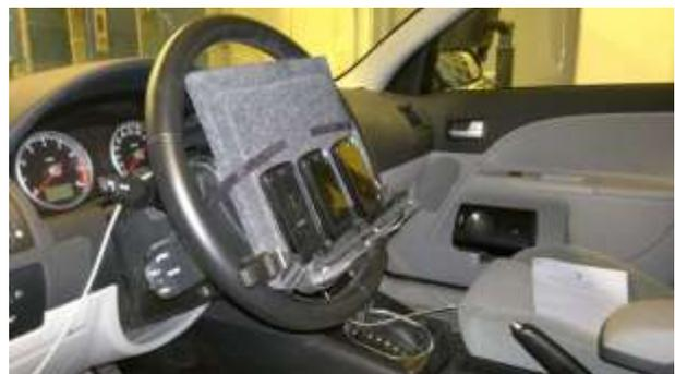
Figure 5: The mobile phones were placed in front of the wheel in the test car.
