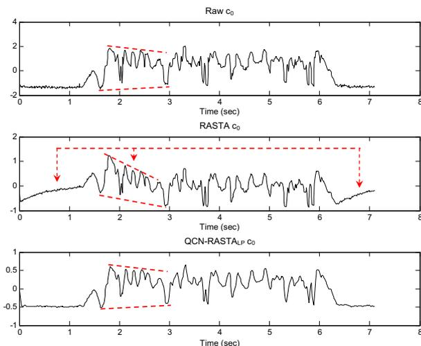
Figure 1: Transient effects due to RASTA filtering – raw, RASTA-filtered, and  $RASTA_{LP}$ -filtered  $c_0$  tracks. Note increased transients due to RASTA filtering (middle plot) compared to  $RASTA_{LP}$ .
