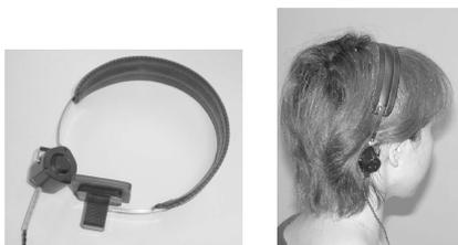
Figure 3: Ceramic vibrator of the BCUHA attached to the mastoid with a hair-band-like device
