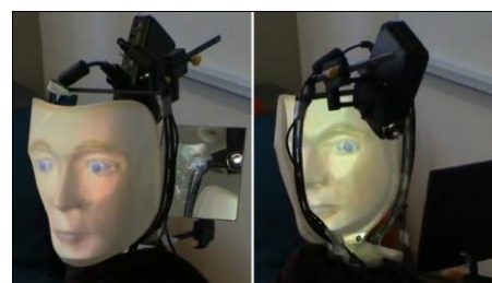
Figure 2. Photographs showing the inner hardware and system rig of Furhat.
