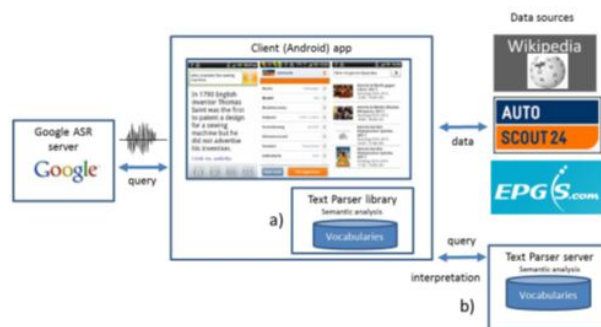
Figure 2: Two possibilities to access rootvole a) on the client, b) as a server implementation
