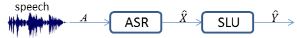
Figure 3: Conceptual process of typical spoken dialog systems with cascaded speech recognition and understanding.
