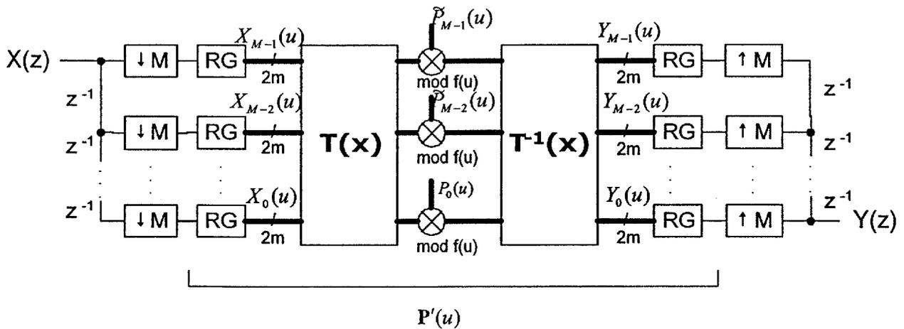
Fig. 3. Digital filter realization in polynomial fields and rings
