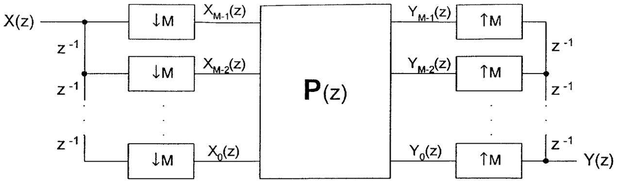
Fig. 1. Equivalent filter bank structure.
