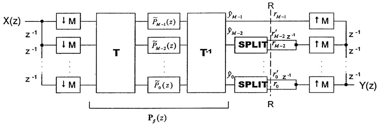
Fig. 2. Digital filter realization by means of MNTT
