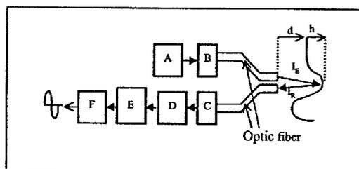
**Figure. 1** Bloc diagram of the Opto-reflectometer
